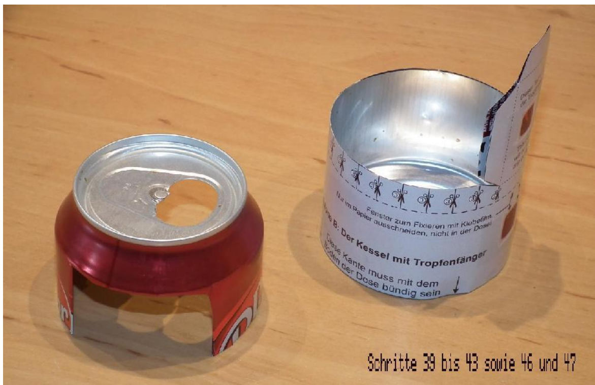
Steps 39 – 43 + 46 and 47: The finished cut-to-size and folded stove (on the left in the picture) and the boiler still being worked on.
